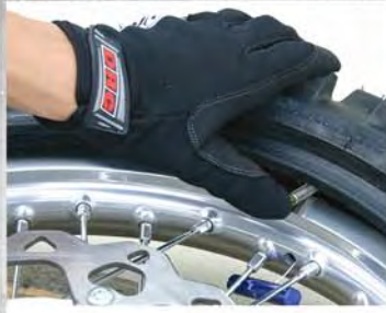
STEP 3: Replace air valve in the tire.
