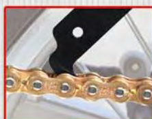
A. Lightly attach Chain checker on the chain roller.
