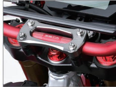
ZE33-2100 COMP Stabilizer W100 ZE58-2123 Stem Nut M24x30-P1.0 H12 Red ZE58-4133 Stem Cap 13-17.5mm Red
