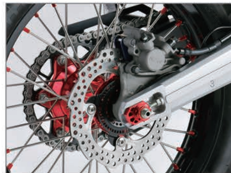
ZE93-8022 Axle Nut M16x27-P1.5 H13L Red ZE93-5063 Rear Axle Block Red W51-20033 Rear DiskRotor SUS
